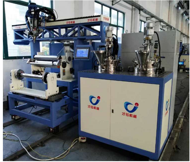
Injection unit – mixing and auto-feeding device
