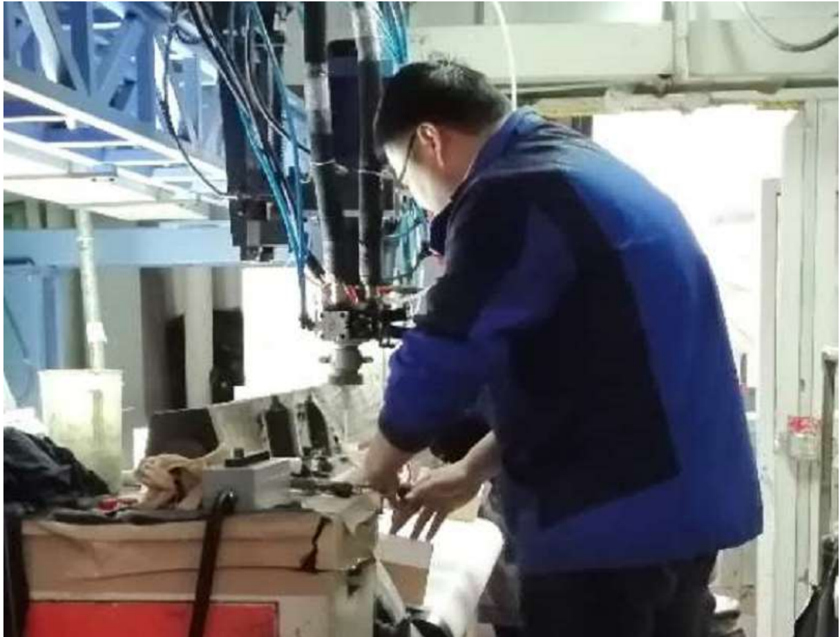
Coating head with automatic feeding unit.
